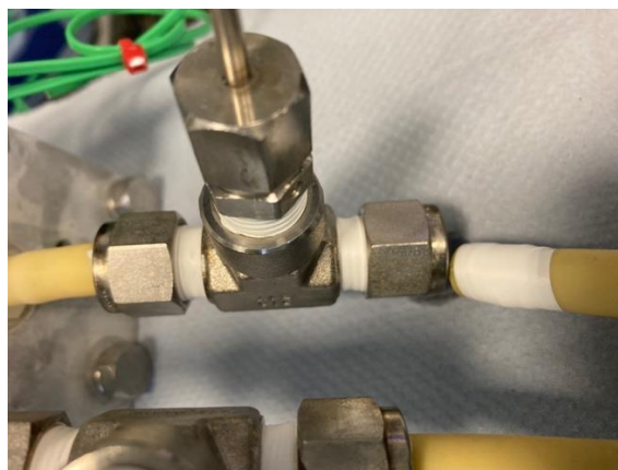
Fig. S1l. Applying PTFE tape to the tubing.
