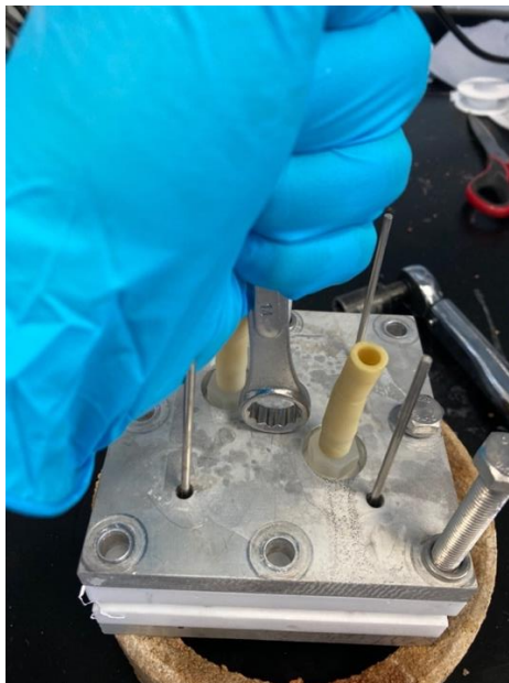
Fig. S1j. Pressing the flow cell down while inserting the hex bolts.
