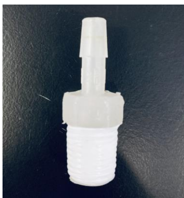
Fig. S1f. Wrapping PTFE tape on the polypropylene hosebarb/fitting.
