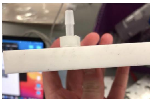
Fig. S1g. The attachment of a tube fitting into a PTFE insulating plate.
